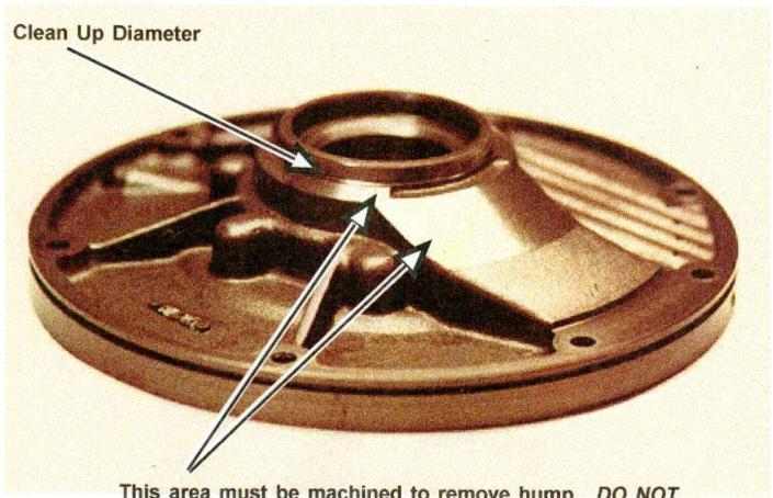
This area must be machined to remove hump. <u>DO NOT</u> machine anymore then necessary to remove hump.
