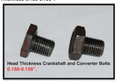
If you do not check this you can tear up the back of the block with the thick converter bolts.
