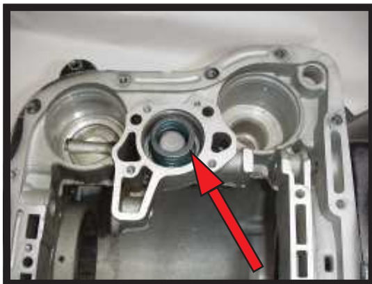
Fig. #3 Remove Spring(s) Do Not Reinstall!
