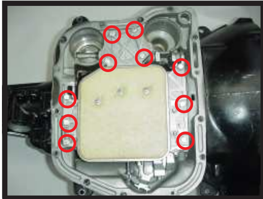
Fig. #1 Remove Ten Bolts
