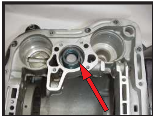
Fig. #3 Remove Spring(s) Do Not Reinstall!
