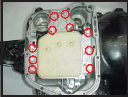
Fig. #1 Remove Ten Bolts
