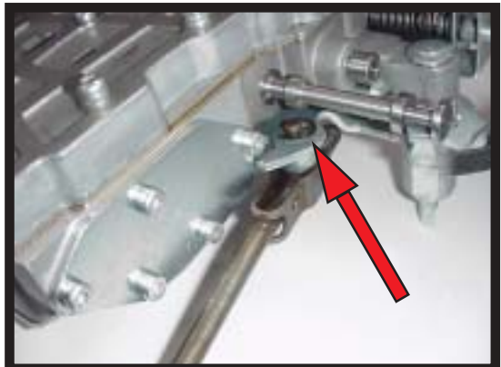
Fig. #4 Remove E-Clip
