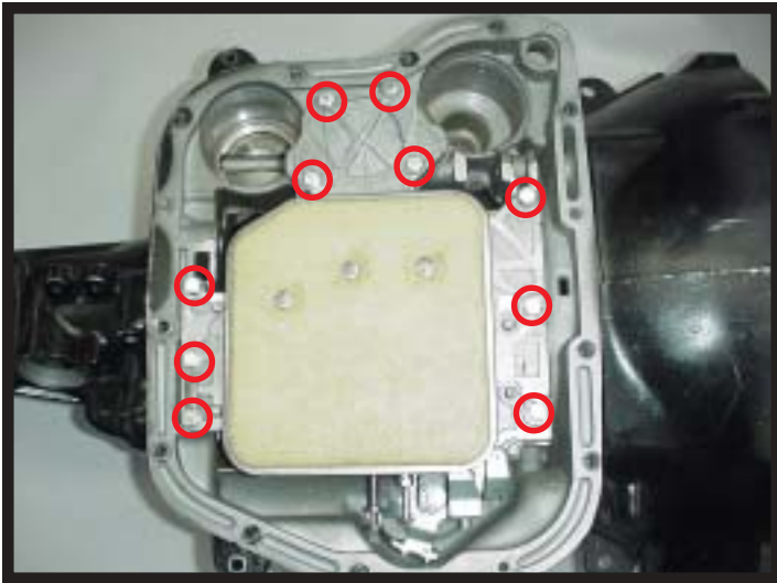
Fig. #1 Remove Ten Bolts
